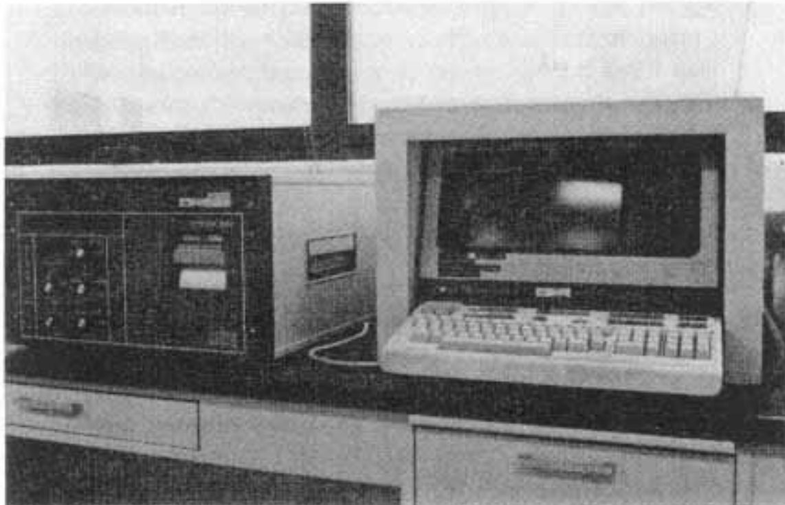
Fig. 2.4 Electronic thermal recording instruments used to monitor rabbit body temperatures during the pyrogen test.
