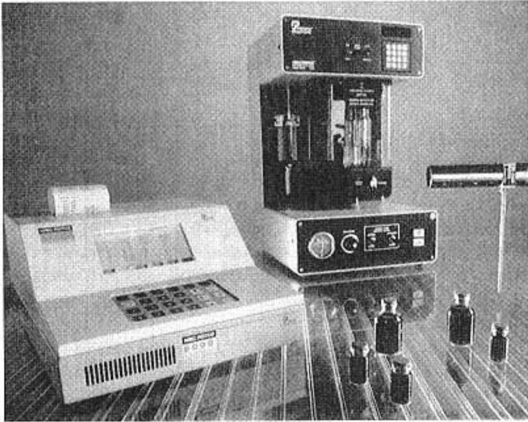
Fig. 3.8 HIAC/Royco's System 8003 for parenteral particle counting to comply with the requirements of USP <788> (courtesy of HIAC/Royco Division of Pacific Scientific Company, Silver Spring, Maryland).
