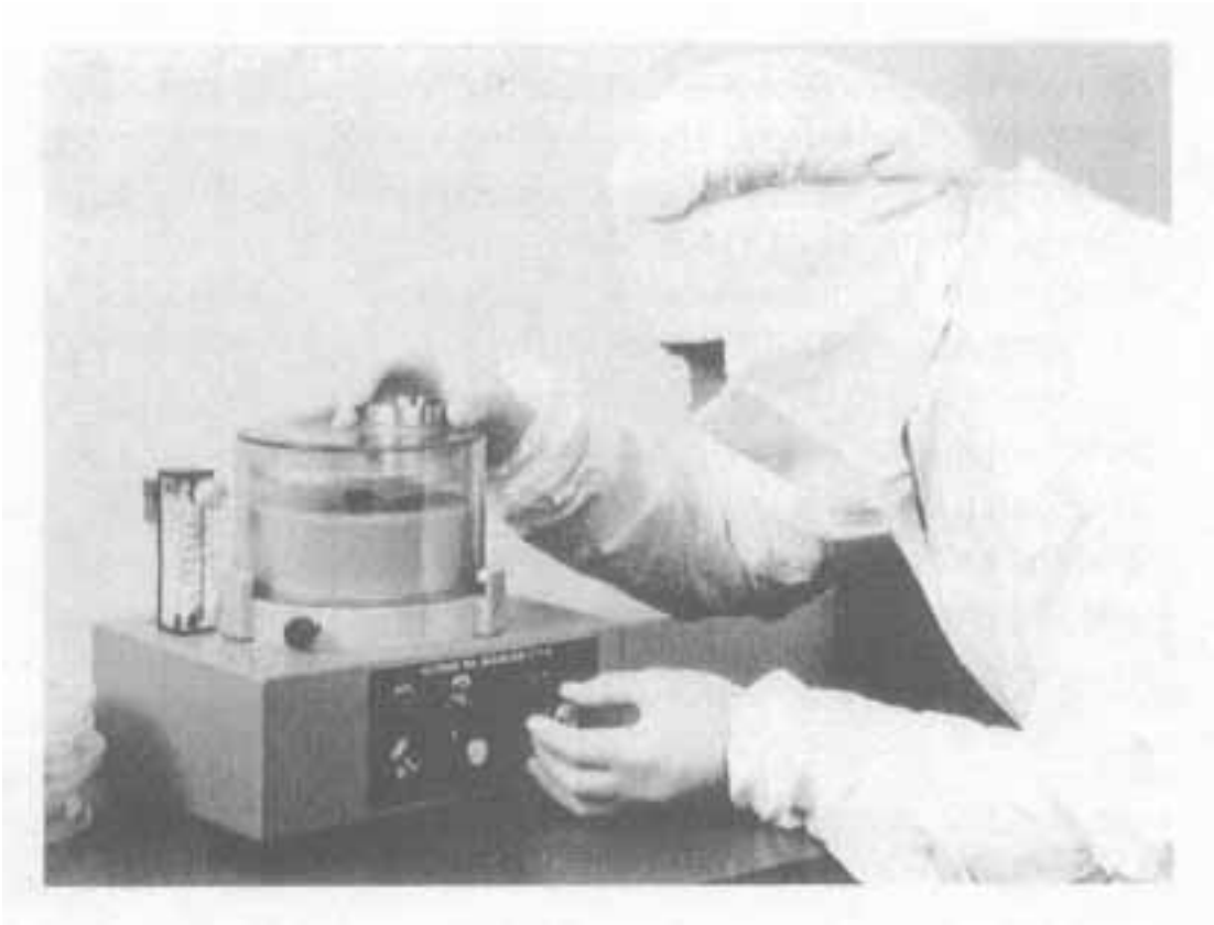
Fig. 1.12 Slit-to-agar biological air sample (courtesy of New Brunswick Scientific Co., Inc., Edison, New Jersey).
